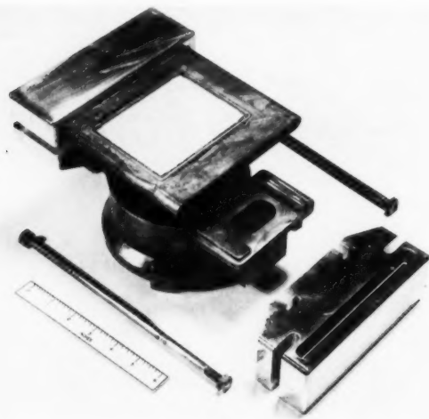
Fig. I-10 High-current flat-plate target partially assembled in header unit.
